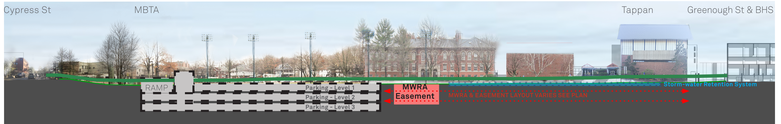
Site Section: Underground Parking Structure Below Cypress Park - Field @ +/- 100 Cars per Level
